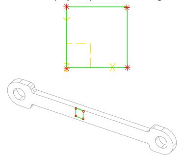
Why: In this example you'll use only one element to understand how nodes and elements behave. The computed displacements and stresses will be correct only for simple uniform loads. In most cases, you'll have to create many smaller elements to converge on a correct result.
