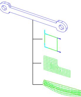
What: Switch to the *Meshing* task and create an FE model.
