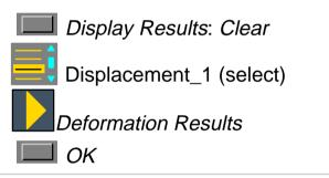
Why: Deformation results will be shown as displaced nodes. Display results are shown in color. By clearing the display results, you can see the displacements more clearly.
