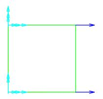
You must apply enough restraints to hold the model as a rigid body in space. Even though the linkage has equal and opposite forces on the two ends, you will restrain one end, and apply a force on the other.
